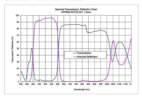
**CLAREX® Near Infrared Cut Filters -** These filters have been designed specifically for NVIS applications where it is important to minimize the amount of NIR light emission. These filters can also serve as NIR-Hot Mirrors.
